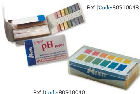
pH paper is a special paper impregnated with an indicator or an indicator mixture that, when put into contact with the solution to be analyzed, adopts a certain colour depending on the pH of this solution. Therefore, pH paper is an economical, simple and very useful method for routine or field pH determinations of aqueous solutions in a matter of seconds. Nahita pH paper is supplied as a strip format (10x70 mm) and in boxes of 200 units each.
